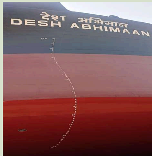
Silicon paint applied on underwater portion of SCI tanker DESH ABHIMAAN
